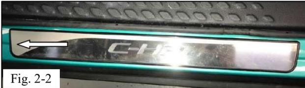
(b) Print and cut the front LH front paper template attached to the document and align it to the vehicle rocker at the start of the inner garnish (Fig. 2-3).
